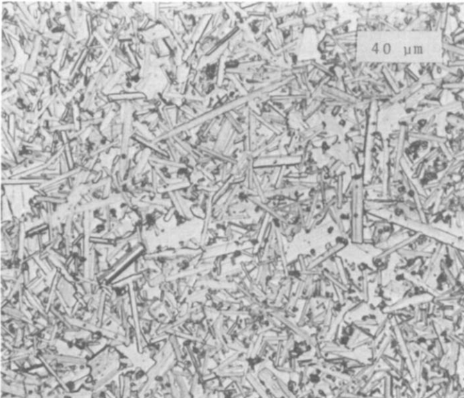
Fig. 3. Etched section of a specimen showing grain size distribution. Note the long tabular \alpha -grains.
